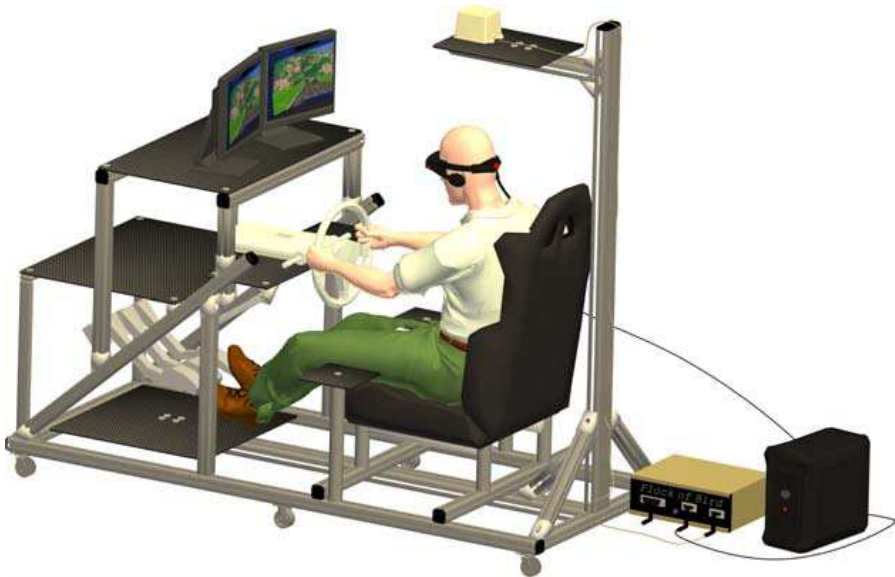
FIGURE 1 Overview of the setup. Participants sat on a playseat integrated into an aluminum frame and wore a head-mounted display. They controlled the velocity of the virtual car with accelerator and brake pedals and lateral excursions between lanes with the steering wheel. Participants' head pitch, yaw, and roll orientations were measured with an electromagnetic tracker and coupled to the visual scene. Participants could also display rear mirrors by pressing buttons on the steering wheel.
